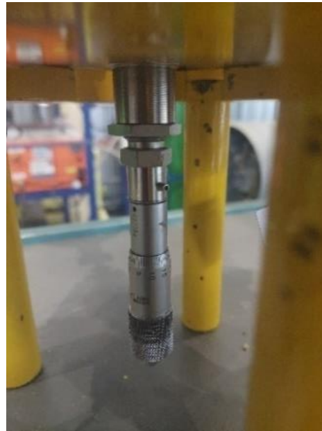
Figure 3.2 Mechanical linear actuator at the bottom of the small-scale vessel to adjust the gap distance between electrodes with a 0.5 mm gap adjustment per revolution.
