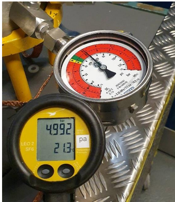
Figure 3.5 Analogue and digital pressure gauges used for monitoring the pressure in the vessel.
