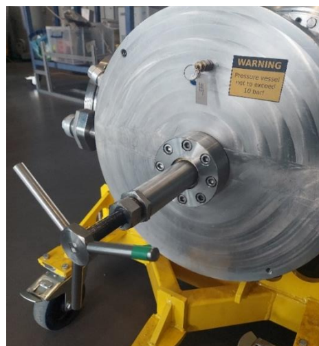
Figure 3.4 Mechanical linear actuator at the side of the large-scale vessel to adjust the gap distance between electrodes with a 1.5 mm gap adjustment per complete revolution.
