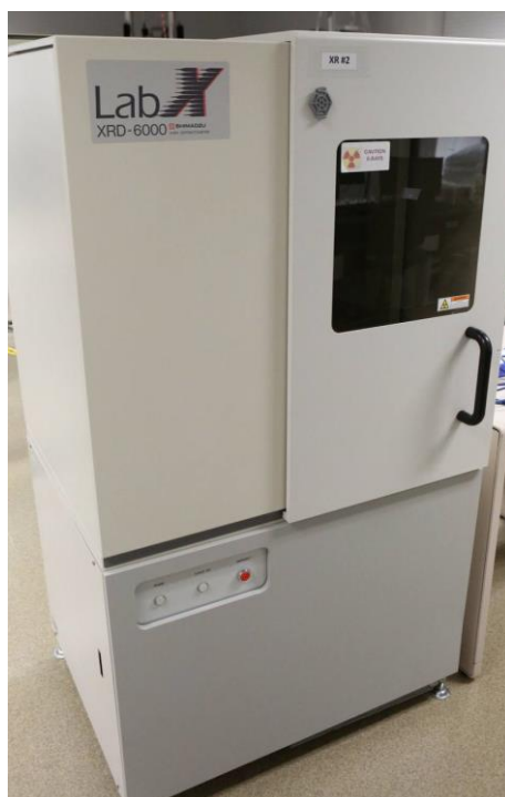
Figure (3.3) X-ray diffractometer Shimadzu 6000 X-ray[46].
